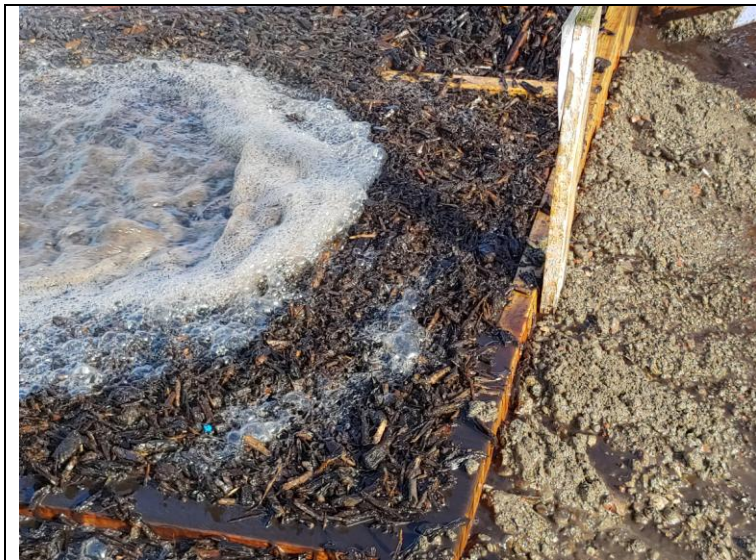
Unscreened Organic Mulch resisting directed water flow
