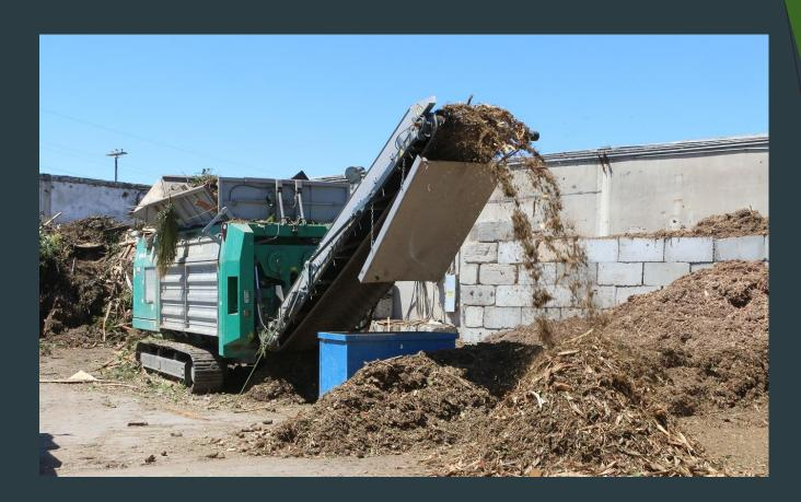
Crambo equipment processing wood and green material into biofuel
