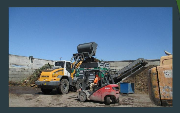
Clean Wood and Green Waste is Loaded into a slow speed shredder for size reduction
