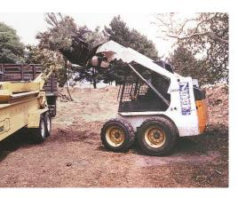
At first, Rubicon staff tried to load all the plant trimmings into the chipper by hand. It quickly became apparent that the staff would not be able to keep up with the grinder. A Bobcat with a grapple bucket is now used to load the machine more efficiently.
