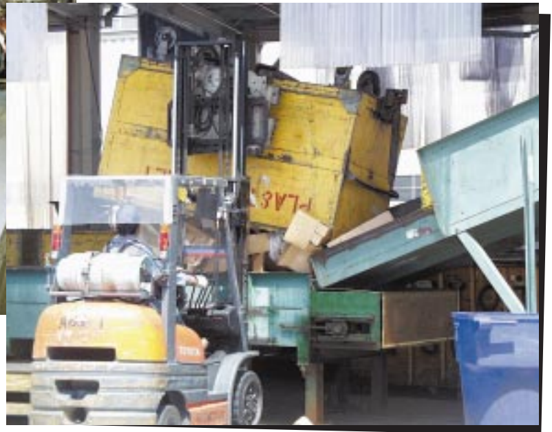
A forklift (right) dumps recyclables onto NUMMI's sorting line which recycles 7,300 tons of material a year.
