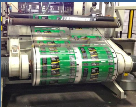
Emerald Packaging's printing press rolling out their biodegradable, plant based PLA.
