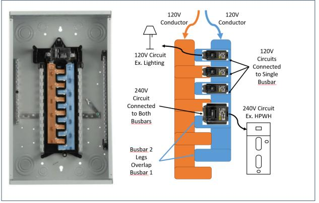
Figure 14. Photograph and Diagram of Inside of a Subpanel (Square D, 2020) (Square D, 2020) (Saltzman) (Murray, 2020)
