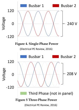
Typically, each supply conductor to a multifamily building is 120 V, so the line voltage between any two supply conductors is 208 V. While a building may be supplied with threephase power, the feeders to the apartments will all be single phase; the only difference to downstream loads is that double-pole circuits will receive 208 V, rather than 240 V.
